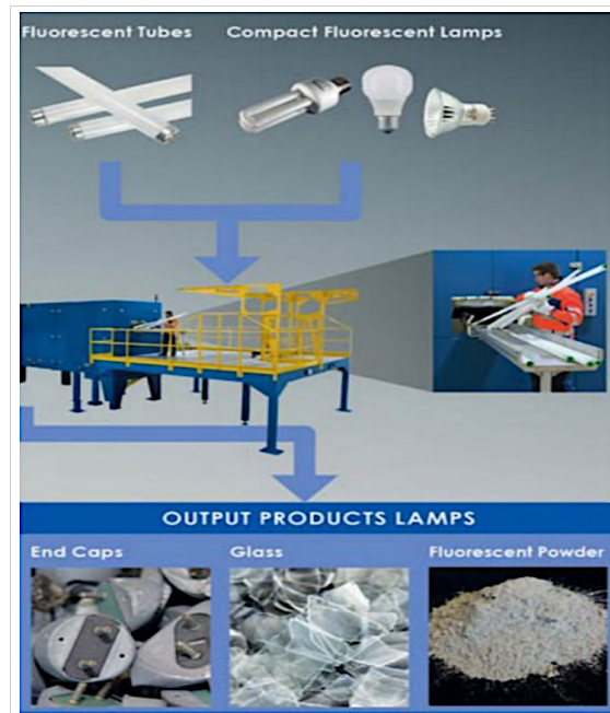
Figure 10: Process flow of lamp recycling by BLUBOX [10].
